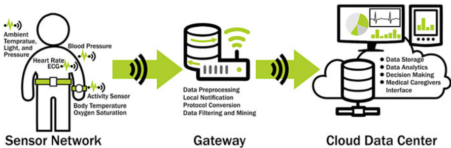
Fig. 8.4 Healthcare IoT system architecture
