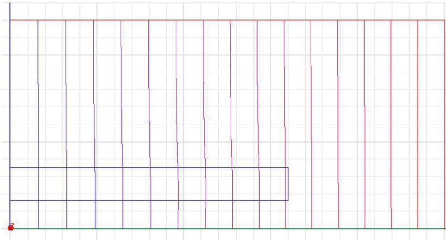
FIGURE 15.13 Flux lines for a stainless steel tie plate in a uniform 60 Hz field of 1 Tesla peak value normal to its surface. The situation is otherwise the same as described in Figure 15.11 .
