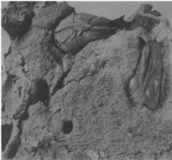
Figure 6.3 Bivalves of the genus Pholadidea in concrete taken from concrete pile jackets off the Californian coast [8].
