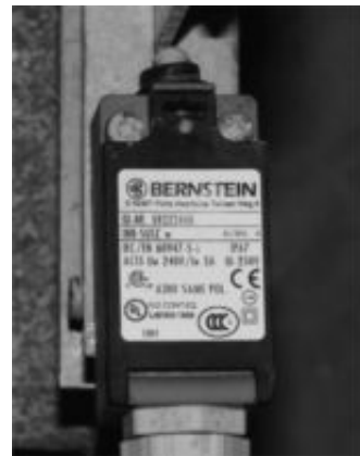
Figure 7. Electrical safety switch.
